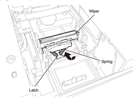
(8) Remove the wiper from the maintenance unit.
