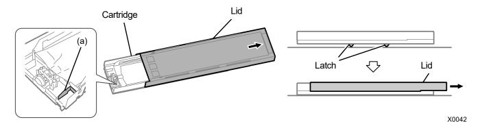
(5) Remove the maintenance solution pouch from the cartridge, and put the white ink pouch in place.
