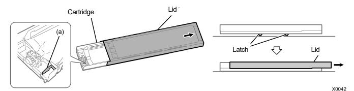
(29) Take out the capping pouch from the cartridge, and put the white ink pouch in place.
