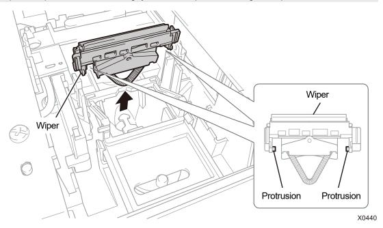
(9) Insert a new wiper into the printer from above.
