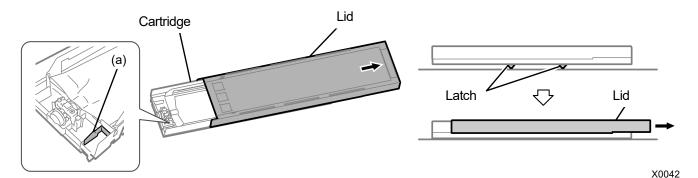
(5) Pinch the latch at the front end of ink pouch, and draw out the white ink pouch from the cartridge.
