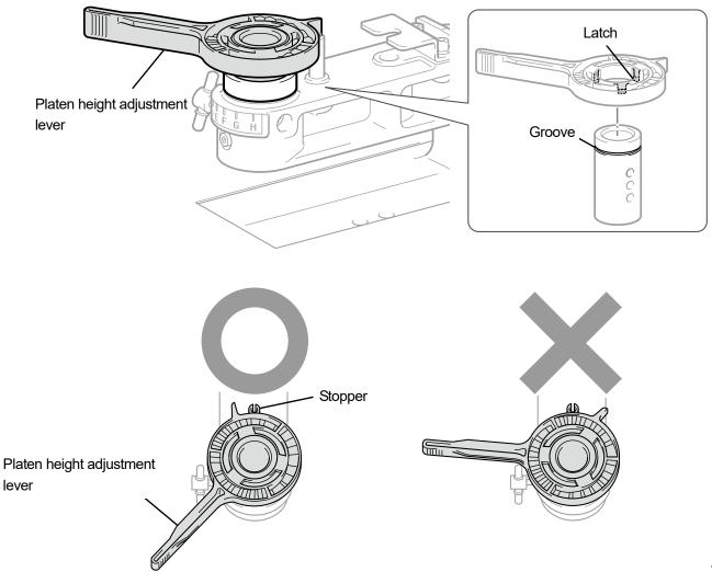
(6) Check that the end position of the platen height adjustment lever is aligned with that of the platen bearing.
