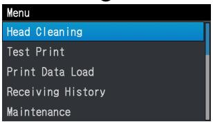
(3) By pressing ▲ / ▼ , select one of the options: [Normal Cleaning], [Powerful Cleaning], [Super Cleaning] or [Flash Firing], and press (CN) .
