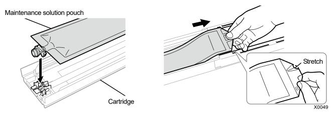
(7) Put the maintenance solution pouch in its correct position.
