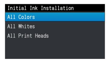
(4) According to the message displayed on the operation panel, press Initial ink installation will be operated.
