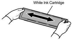
Shake 100 times (for approx. 50 seconds) (Swing distance should be approx. 2 in. (5 cm). Increase the swing distance when the remaining ink level becomes low.)
