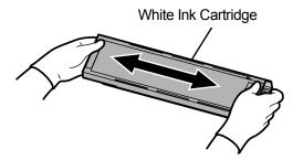
Shake 100 times (for approx. 50 seconds) (Swing distance should be approx. 2 in. (5 cm). Increase the swing distance when the remaining ink level becomes low.)
