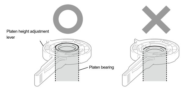
(5) Loosen the knob while holding the platen height adjustment lever and lower the platen bearing and the height control lever.
