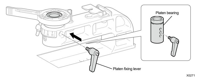
(9) Tighten the knob to secure the platen bearing in place.
