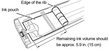
(8) Open the lid of the cartridge and place the ink pouch in its correct position.
