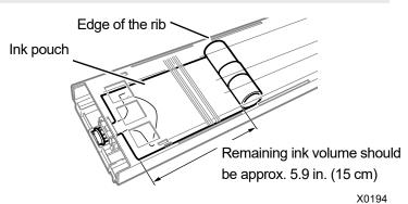
(32) Open the lid of the cartridge and place the ink pouch in its correct position.
