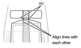
Place the pouch in a straight alignment with the cartridge
