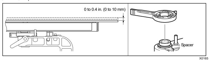
As an example, the cases where the platen's height is set to the lowest position from the standard position and to the middle position from the lowest position are described below.
