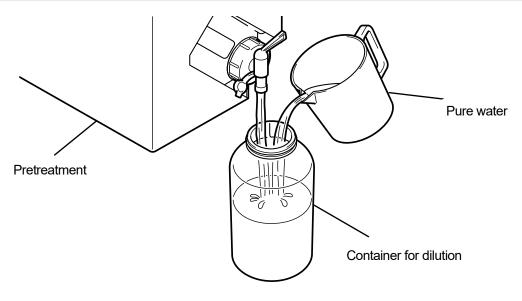
(5) To provide safekeeping for the pretreatment, close the faucet, place the pretreatment with the faucet part facing upward, and store the entire carton in a safe place.
