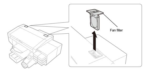
(6) Mount a new fan filter to the frame of filter case.
