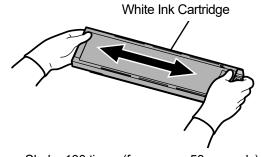
Shake 100 times (for approx. 50 seconds) (Swing distance should be approx. 2 in. (5 cm). Increase the swing distance when the remaining ink level becomes low.)
