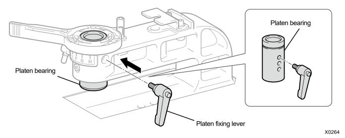
(7) Tighten the knob to secure the platen bearing in place.
