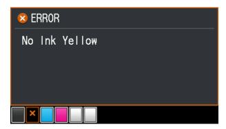
(1) Take out the ink cartridge displayed on the screen from the printer.
