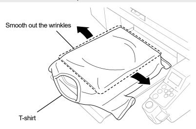
(5) The T-shirt should be placed on the T-shirt tray, trying not to draw the excessive parts like sleeves and hems into the printer.
