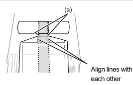
Place the pouch in a straight alignment with the cartridge
