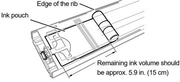
(3) Open the lid of the cartridge and place the ink pouch in its correct position.
