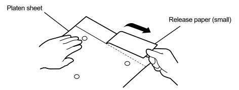
(6) Position the platen sheet to match the platen surface, and onto the platen, stick the portion of the platen sheet where the release paper (small) was removed.
