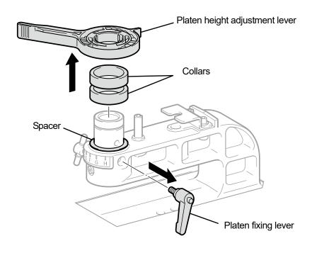
(3) Attach the platen height adjustment lever to the platen bearing.
