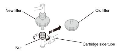
(11) Attach the cartridge side tube to a new filter and fasten the nut.
