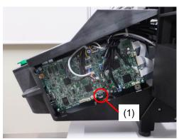
(2) Remove the Lithium Battery (1) by pulling out the holder in the direction of the arrow.
