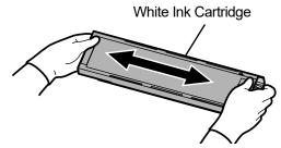
Shake 100 times (for approx. 50 seconds) (Swing distance should be approx. 2 in. (5 cm). Increase the swing distance when the remaining ink level becomes low.)
