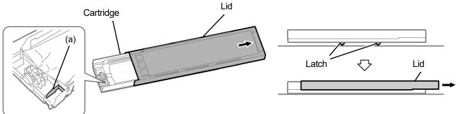
(4) Take out the maintenance solution pouch from the cartridge, and put the white ink pouch in place.
