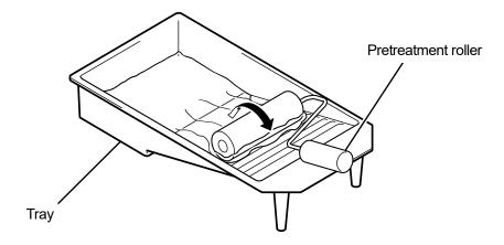
(7) Move the pretreatment roller on the T-shirt in a longitudinal direction, and apply the agent evenly onto the print range.
