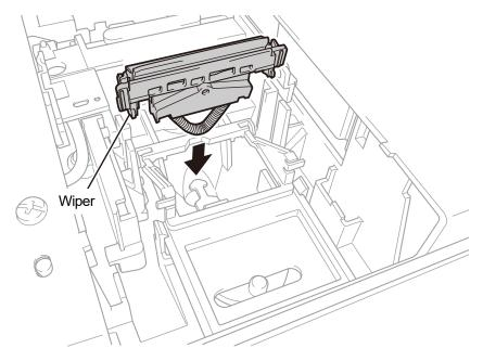
(10) Place the spring under the wiper on the maintenance unit latch.
