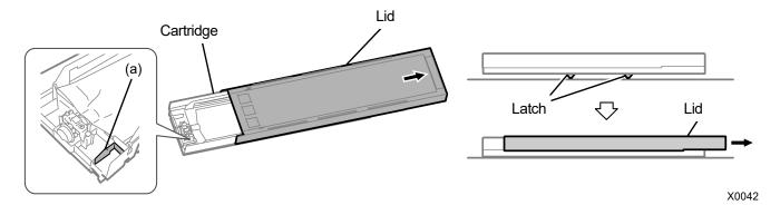
(5) Pinch the latch at the front end of the ink pouch, and draw out the white ink pouch from the cartridge.
