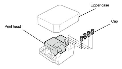
(6) Remove each tube from the print head to be replaced with a new one, then attach each of the new caps which are removed from a new print head to each tube, while exercising care to prevent any ink from being spilled.
