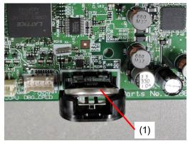
(3) Pickup the Lithium Battery (1) to the direction of the arrow.
