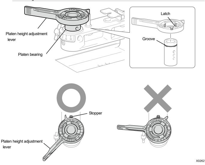
(4) Check that the end position of the platen height adjustment lever is aligned with that of the platen bearing.
