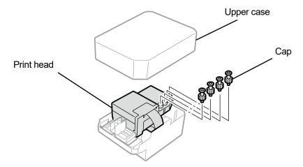
(7) Remove each tube from the print head to be replaced with a new one, then attach each of the new caps which are removed from a new print head to each tube, while exercising care to prevent any ink from being spilled.
