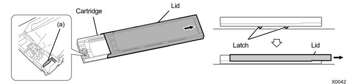
(3) Pinch the latch at the front end of ink pouch, and draw out the depleted ink pouch from the cartridge.
