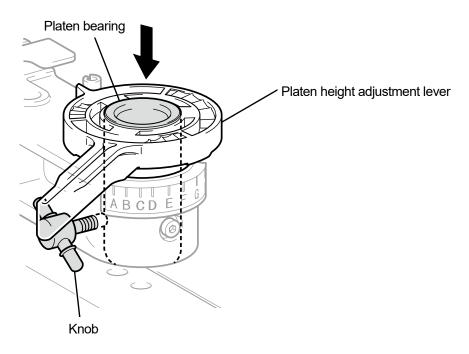
(8) Use the platen fixing lever to secure the platen temporarily.
