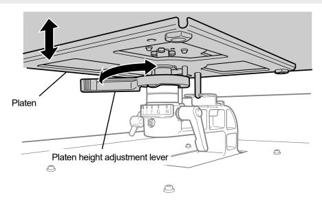
(3) Put a T-shirt onto the platen, with its printing side facing upward.
