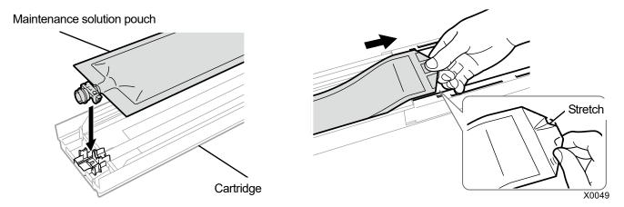
(7) Put the maintenance solution pouch in its correct position.
