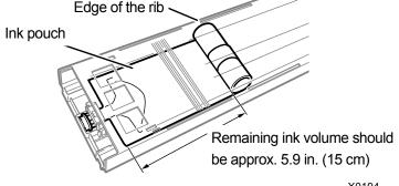
(7) Open the lid of the cartridge and place the ink pouch in its correct position.
