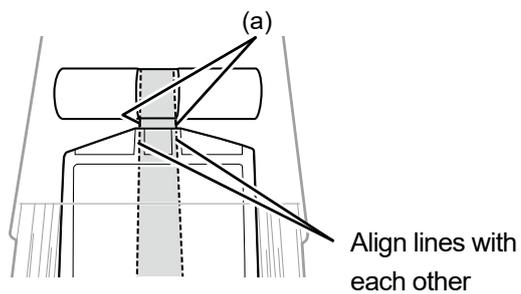
Place the pouch in a straight alignment with the cartridge
