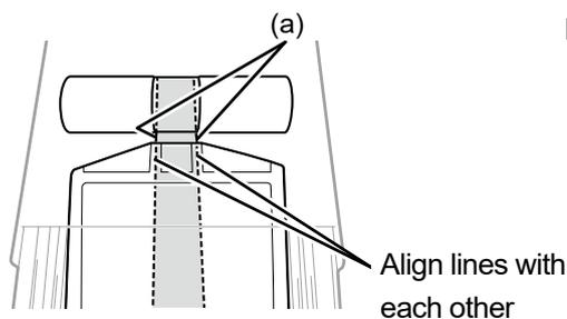
Place the pouch in straight alignment with the cartridge
